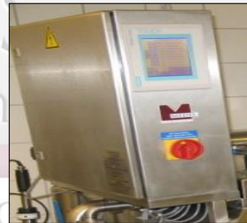
MA-1500 P.E.G. Infiltrator with integrated touchscreen programming
