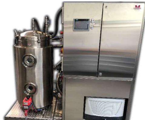
Bone fat extraction system with DCM recovery and Bone degreasing module. Degreasing chamber: 500mm AD x 900mm(H)
