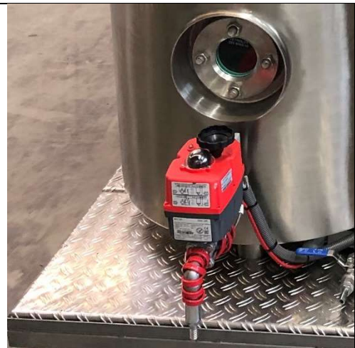
Heated outlet for bone fat on the front of the unit. Easily accessible and effective
