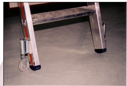
Locking mechanism of the safety ladder
