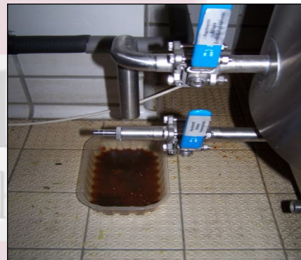
Heated outlet for bone fat sideways for easy access and effectivity. A closed system reservoir is standard!
