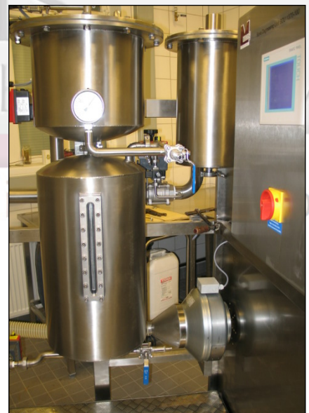
MA-1390 Dichlormethane (DCM) – recycling unit with condenser and storage tank of reusable DCM
