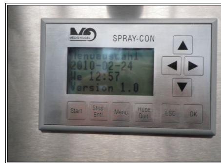
SprayCon control unit with display and visual and acoustic alarm. All messages in English language
