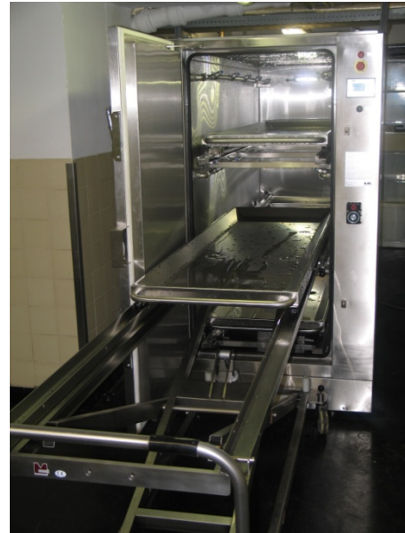
Automatic loading / unloading of the SprayCon unit
