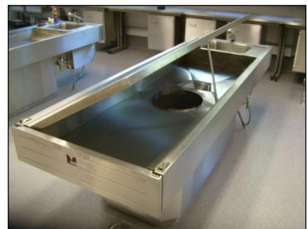
example of a so-called "dom" suction, which we made as a special version only once. Have. The floor is not smooth and the exhaust air pipe goes directly into the exhaust air system. Our
