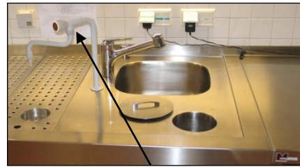
Manual formalin tap for fresh formalin mounted to a MEDIS MT Tissue Grossing Station MA-0032.
