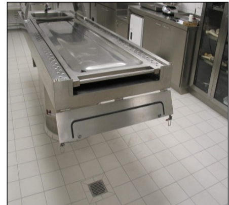
Transfer lid opened after insertion of roll on / roll off work area (body tray)
