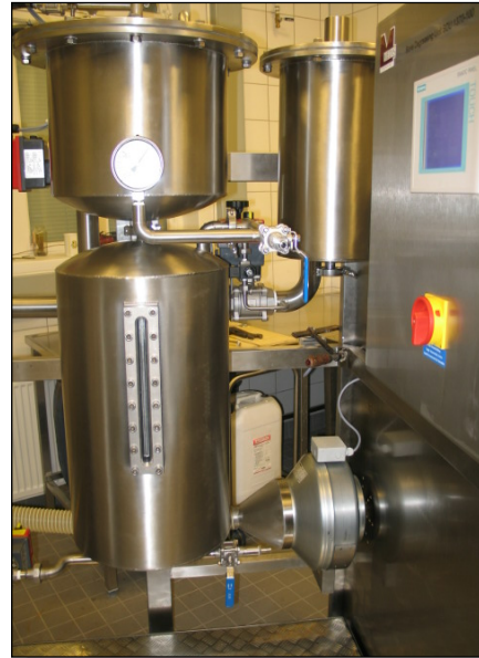
Dichlormethane (DCM) – Recycling Unit with condenser and storage tank of reusable DCM.
