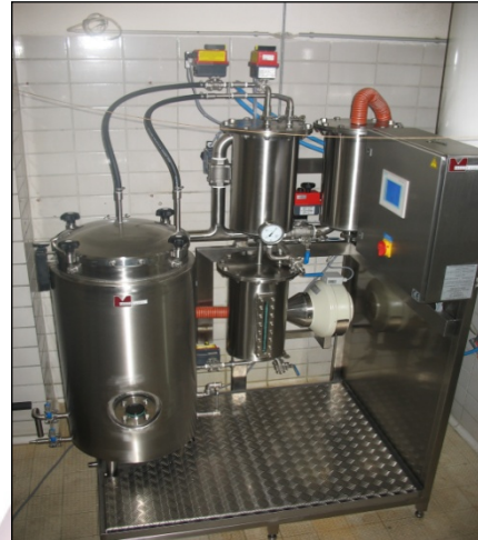
BDU-1370-50 Bone Fat Extraction Unit with DCM-recycling and bone drying modules Degreasing chamber size: 500mm AD x 900mm(H)
