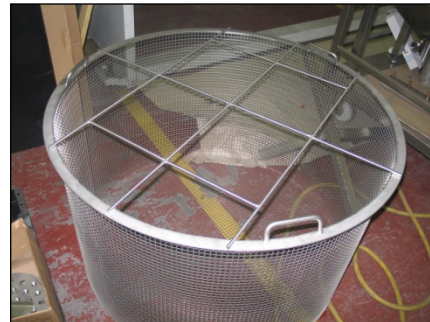
Process basket with rods for specimen hooks
