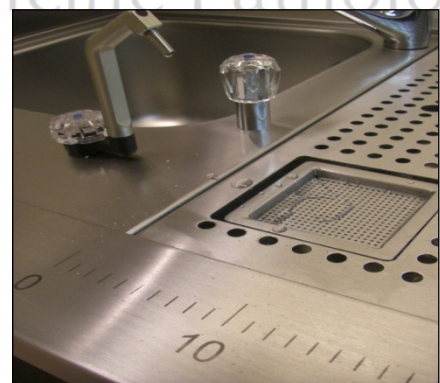
c Station with formalin waste drain covered by a fine screen, fresh formalin dispenser and graduation
