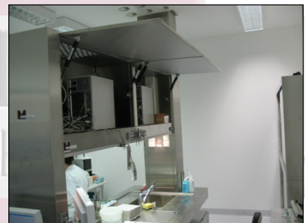
Superstructure for accommodation for PC, camera etc.
