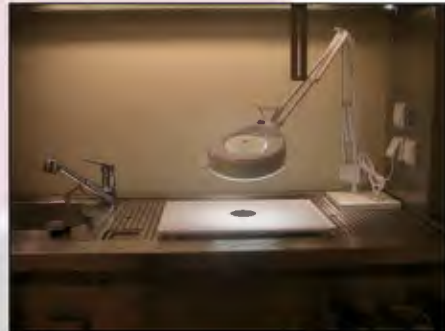
MA-0880 MacroDoc Station with magnifier lamp, grossing board with black orientation field and holder for camera
