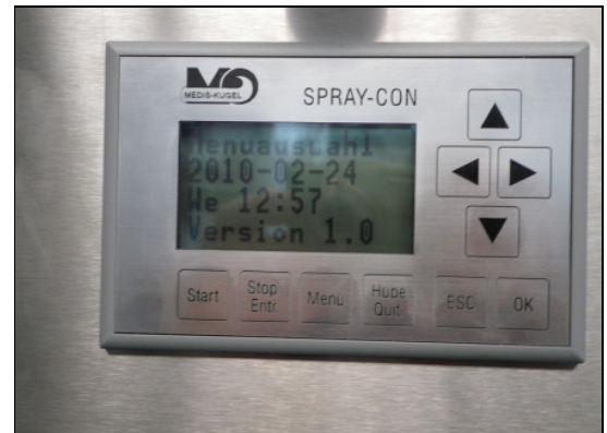
SprayCon contro unit with display and visual and acoustic alarm. All messages in english language.
