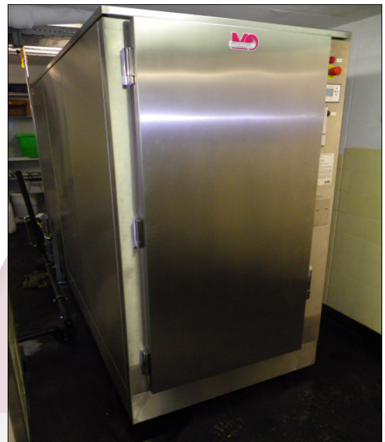
MA-5000 SprayCon© CS Module in operation. Totally closed system.
